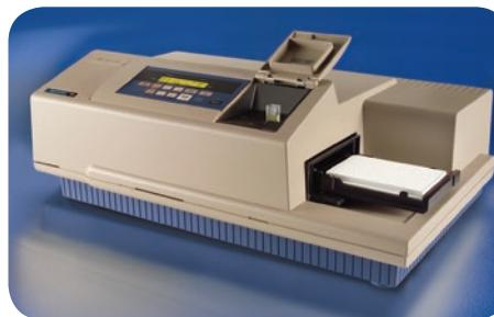
Upgradeable platform; tunable absorbance, fluorescence, luminescence; TRF (M4 only), triple-mode cuvette port, kinetics, spectral and well scanning, AutoPMT™, PathCheck®
