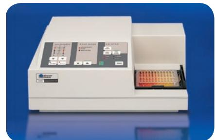
Filter-based (visible 405-750 nm) endpoint, 96-well (kinetics on VMax)
