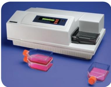
Tunable (250-850 nm), fluorescence, top-and bottom-read, cell-based assay, FRET
