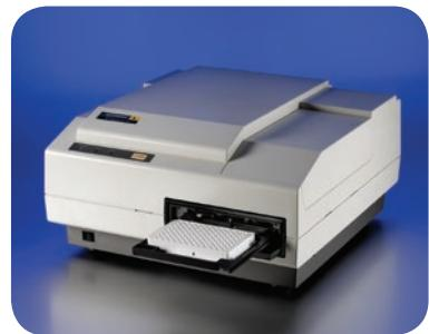
Up to 6-times faster, > 9 orders of dynamic range, dual injection in both 96- and 384-well microplates, excellent sensitivity, Autorinse injectors, optional BRET configuration
