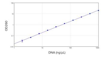
The SpectraMax iD5 reader is fully compatible with the SpectraDrop<sup>™</sup> Micro-Volume Microplate, enabling quantitation of precious low-volume samples. 4-µL DNA standards from 2 ng/µL to 1000 ng/µL were read in absorbance detection mode with a preconfigured protocol in SoftMax Pro Software. Performance matching the 2 ng/µL sensitivity specification is demonstrated here.
