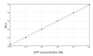
An ATP standard curve spanning five decades was run using the ATPlite 1step Luminescence Assay System (PerkinElmer) on the SpectraMax iD5 reader. Standard concentrations ranged from 1x10<sup>-11</sup> M to 1x10<sup>-6</sup> M. A wide linear dynamic range ensures accurate assay results across a broad span of sample types. Standards were plotted using a log-log curve fit in SoftMax Pro Software.
